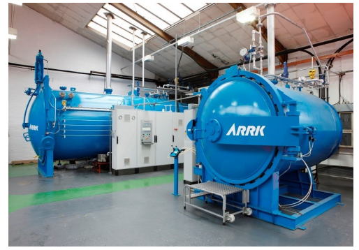
Large Autoclaves, used in the production of our composite components
