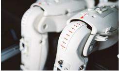
Parts ranged in size and complexity from the dummy's head, torso, arms and hands, through to its legs and feet. Numerous SLS parts also needed to be joined, assembled and re-enforced with glass fibre matting to provide additional strength. The prototyping team were also required to source, manufacture and incorporate over 60 CNC machined components in steel and aluminium. These parts also included some welded fabrications, before being fitted inside the SLS parts by the Gloucester team.
